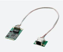
NISKLAN03 without bracket, cable length 250mm (P/N: 10JKLAN0300X0)
